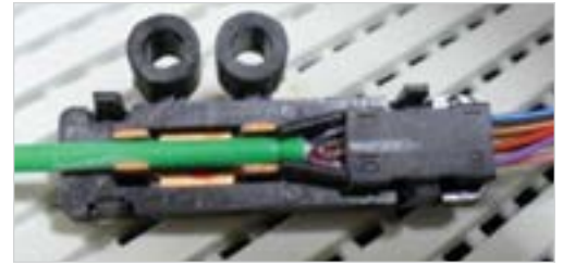
Fiber loose tube crushed in breakout kit
