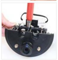
5.4 Remove the solid grommets and select the appropriate sized loop-thru grommets (square outer sides) and place in center ports. Cut a slit completely through one side of the grommet with splicing scissors and place cable through the slit. Repeat for the other port on the opposite side.
