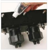
7.5 Assemble the base tightly, using a 216C tool. Reattach cable clamps. Reinstall the main closure gasket.
