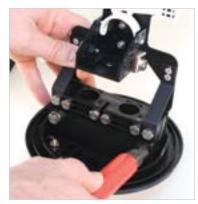
3.3 Slightly bend the bolt side of the base downwards to release it from the locking tabs located on the underside. Pull the two sections apart.
