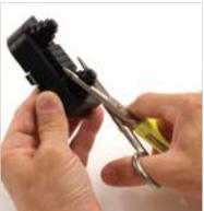
6.4 Because the cable cannot be pushed through the end grommet on loop-thru applications, the end grommet must be cut from its top side to install the cable. Remove the metal bar and retaining ring (2 halves).
