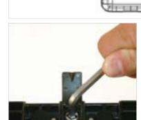
2.3 For opening the Type A closure, loosen and disengage all eight (8) captive 7/16" hex bolts with the 216C tool to remove the upper closure cover.
