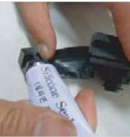
6.8 Place cable through the cut in the top side of end grommet and reinstall the metal bar and retaining ring halves to the grommet. To ensure a weatherproof seal, a cable tie should be tightly fastened around the concentric hole of the end grommet and cable.
