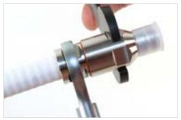
11. Until connector is ready for use, leave plastic cap on connector end to prevent contamination. Installation is complete.
