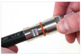
9. With a 21 mm open end wrench, hold connector top in place. Thread connector base to connector top and tighten with a 19 mm torque wrench set at 15 ft-lbs. A 22 mm open-ended wrench should be used for holding the connector top when tightening right angle connectors to the base. The O-ring should no longer be visible and the connector should be tight.
