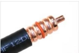
5. Apply provided grease on O-ring and spread evenly.
