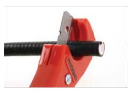
Insert straightened cable end into prep tool, start drill and apply steady pressure until cut material is discharged and you hear and feel a change in drill speed. Maintain tool rotation while removing the tool from the cable.
