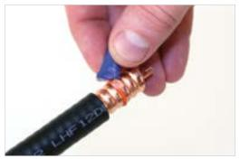
Push connector base onto cable until connector base locks over first corrugation. The outer conductor of the cable should protrude slightly past the connector base.
