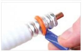
Push connector base onto cable until connector base locks over first corrugation. The outer conductor of the cable should protrude slightly past the connector base.
