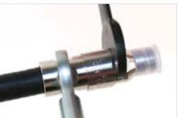
Until connector is ready for use, leave plastic cap on connector end to prevent contamination. Installation is complete.
