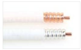
4. Trim dielectric so that it is even with the outer conductor.
