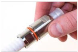
10. With a 21 mm open end wrench, hold connector top in place. Thread connector base to connector top and tighten with a 19 mm torque wrench set at 15 ft-lbs. A 22 mm open-ended wrench should be used for holding the connector top when tightening right angle connectors to the base. The O-ring should no longer be visible and the connector should be tight.
