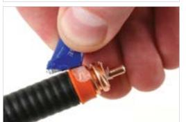
5. Using a 19 mm wrench, thread the connector base until one full corrugation spiral is exposed beyond the connector end (1/4 inch or 2.5 mm).
