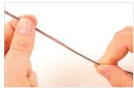
4. Hold the folded ribbon with one hand and position the forefinger of the other hand between the two 12-fiber unit splits. With a unit on either side of the forefinger, use your thumb to hold the outside unit in place and run the forefinger the length of the creased ribbon. The ribbon should separate cleanly.
