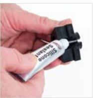
6.9 Place cable through the cut on the bottom side of end grommet. To ensure a weatherproof seal, a cable tie should be tightly fastened around the concentric hole of the end grommet and cable. Use black silicon sealant to seal any additional gaps in the grommet.
