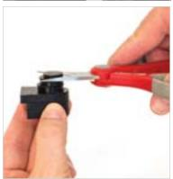
6.6 Because the cable cannot be pushed through the end grommet on loop-thru applications, the end grommet must be cut from its top side to install the cable. Using a razor knife, make a clean cut from the top side of the grommet to the cable entry hole.
