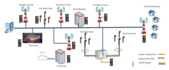
Fiber cable is common to all 5G deployments. There are three different methods for building a 5G network, depending on the type of spectrum in which a wireless carrier has invested.
