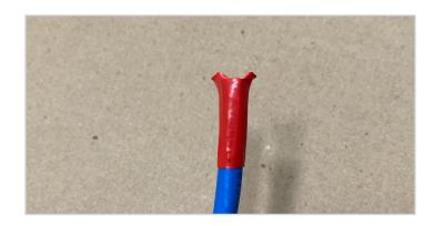
iii. Wrap tape several times around the circumference of the cable over the first two pieces of tape to prevent the tape from snagging and potentially pulling loose during installation.
